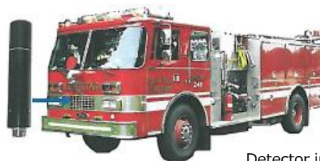
Detector in Engine Compartment
